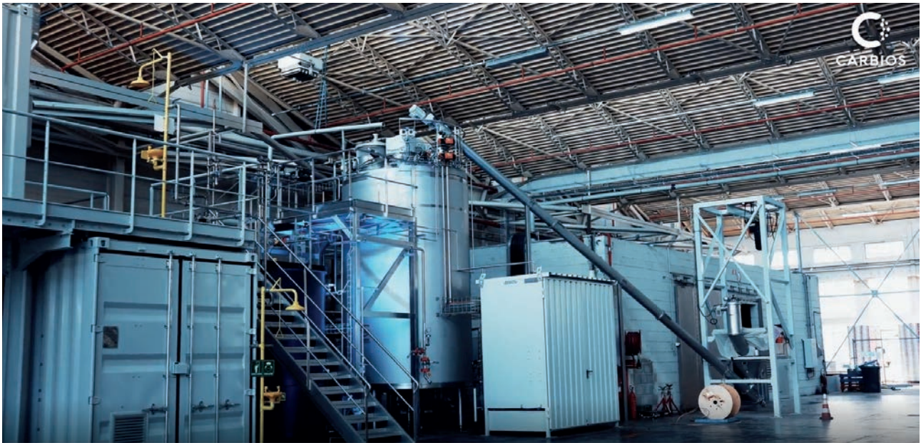
Carbios industrial demonstration plant for the depolymerization of PET plastic waste and textiles into monomers. (Carbios)
