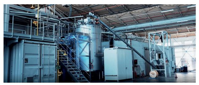
Enzymatic hydrolysis reactor for the depolymerization of PET plastic and textile waste into monomers (credit: Carbios)
